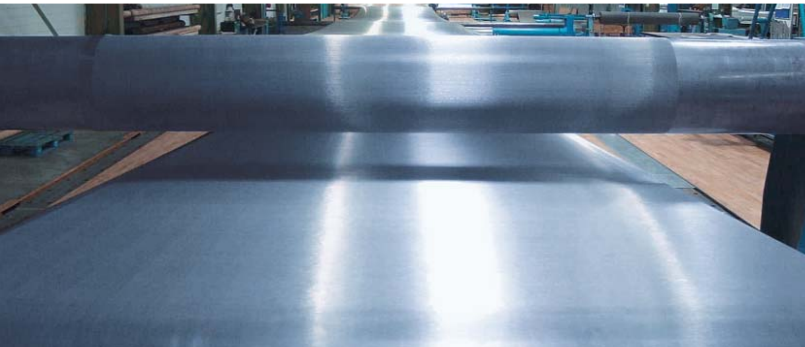
Stretching machine: guarantees absolute flatness of the metal woven belts
